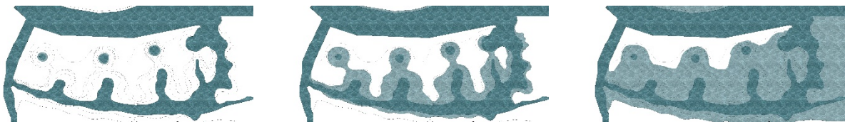
Figure 5: Gdańsk case study - water level rise adaptability. Simulation of the ability to accommodate rising water levels without compromising the designed land development, thanks to the use of elevations and floating and amphibious architecture (modelling and graphics by J. Gorzka).
